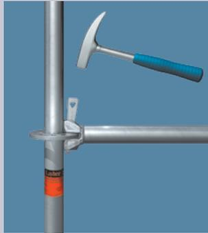
A hammer blow on the wedge transforms the positive connection into a non-positive one. The end face of the wedge head is now positioned precisely at the standard.
