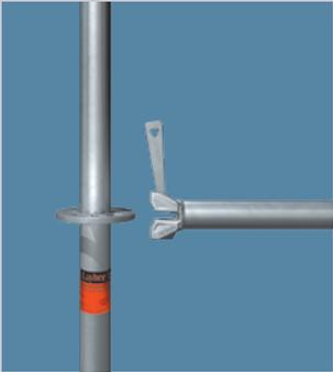
Allround equipment features a simple, unique and bolt-free connection technology. When the wedge head is pushed over the rosette, the wedge drops automatically into the recess thanks to the innovative AutoLock function and is immediately secured against being moved or falling out.
