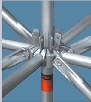
The result of superior engineering. Up to eight connections can be made in the structurally ideal Allround connector, on one level and at various angles. Attachment is possible at the standard dimension intervals of 50 cm on all Allround standards. The flat rosette prevents clogging by dirt of any type.
