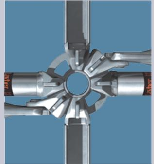
Ingenious connection technology. The four small punched-out openings in the rosette automatically centre the ledger at right angles – the four large openings permit alignment with free selection of the angle.
