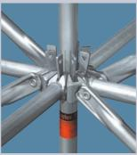
Up to eight connections can be made in the structurally ideal Allround connector, on one level and at various angles. Attachment is possible at the standard dimension intervals of 50 cm on all Allround standards. The flat rosette prevents clogging by dirt of any type.
