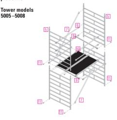
During erecting and dismantling, system decks or scaffolding planks according to DIN 4420 (minimum dimensions 28 x 4.5 x 250 cm long) must be installed as auxiliary decks at heights of max, 2.0 m. These auxiliary decks provide firm footing for erecting and dismantling and must be removed after assembly is complete. The full deck area must be boarded over.
