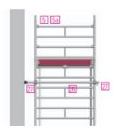
For work performed on a load-bearing wall, ballasting can be reduced in accordance with the ballasting table (see p. 7).
