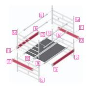
After attaching the top ladder frames 5 or 5 and securing them with spring clips 111 an access deck 10 and deck 9 are suspended from the 5th rung from the top. The regulation side quard is provided by installing two double guardrails 8 or four single guardrails 6. Place two toe boards 12 between the ladder frames 5 and secure them by inserting two 1 44 m end toe boards 13
