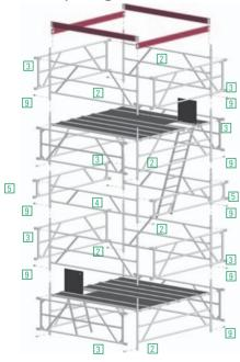
During assembly and dismantling, system decks or scaffold planks according to DIN 4420 (minimum 28 x 4.5 x 350 cm long) must be built in as auxiliary decks at maximum height intervals of 2.0 m. These auxiliary decks, providing a safe footing for assembly and dismantling, are removed after the erection.
