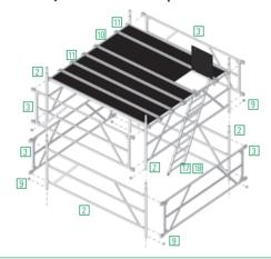
During assembly and dismantling, system decks or scaffold planks according to DIN 4420 (minimum 28 x 4.5 x 350 cm long) must be built in as auxiliary decks at maximum height intervals of 2.0 m. These auxiliary decks, providing a safe footing for assembly and dismantling, are removed after erection. Each platform must be completely boarded.
