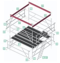
The top platform has to be completely boarded with decks [11] and one access deck [10]. Take care that the horizontal gap between the decks does not exceed 25 mm.
