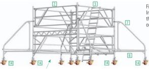
Fix the outrigger \( \bar{2} \) to the plug-in frame \( \bar{2} \). Insert the castors \( \bar{14} \) into the outrigger \( \bar{2} \) and secure them against falling out by fastening the wing screws on the spindle nuts.
