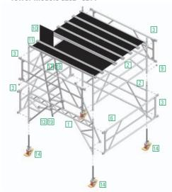
For tower models 8202-8214 access-frames  $\boxed{1}$  1.95 m/2.8 m, plug-in frames  $\boxed{2}$  1.95 m/2.8 m and bracing elements  $\boxed{3}$  1.95 m/2.8 m are built in. These rolling towers differ in their platform size (see assembly examples on page 2). The first access frame  $\boxed{1}$  and plug-in frame  $\boxed{2}$  are connected with two bracing elements  $\boxed{3}$ . Do it by clipping the snap-on claws onto the plug-in frame  $\boxed{2}$  and the access frame  $\boxed{1}$ .
