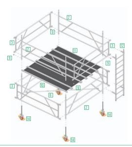
The tower model 8201 has a platform size of  $2.8 \times 2.8 \text{ m}$  and is built-up with plug-in frames 2.8 m and bracing elements 2.8 m.
